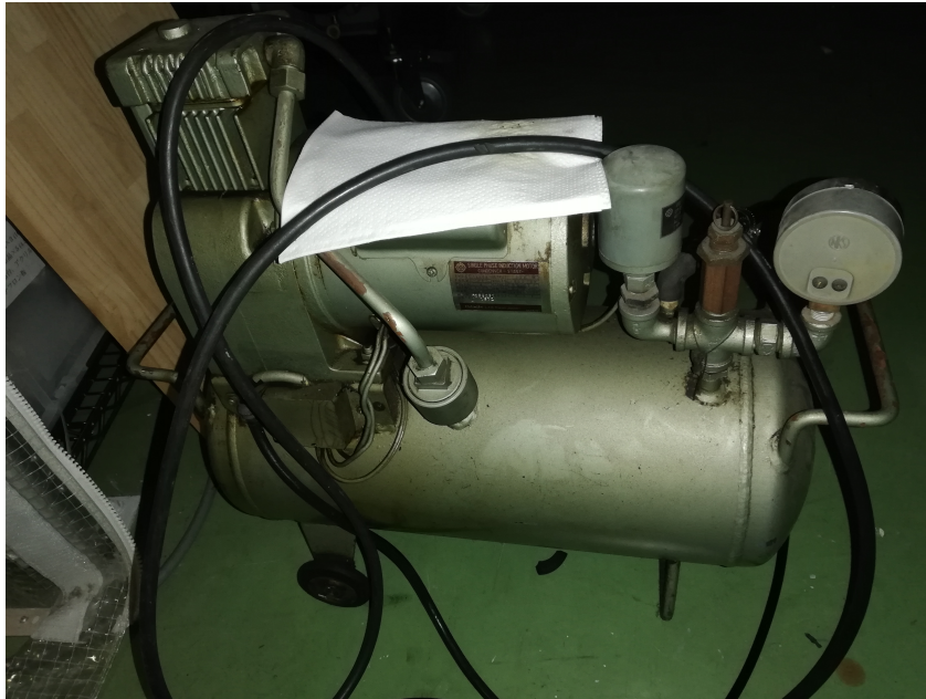
Figure 4.9: Air compressor for the external TMP pump.
