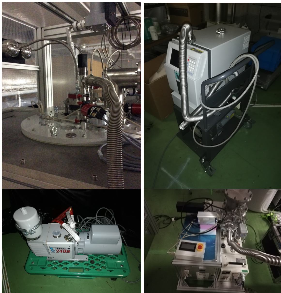
Figure 3.5: From top right to bottom left:- OVC valve, Helium Leak Detector, Rotary pump, TMP unit
