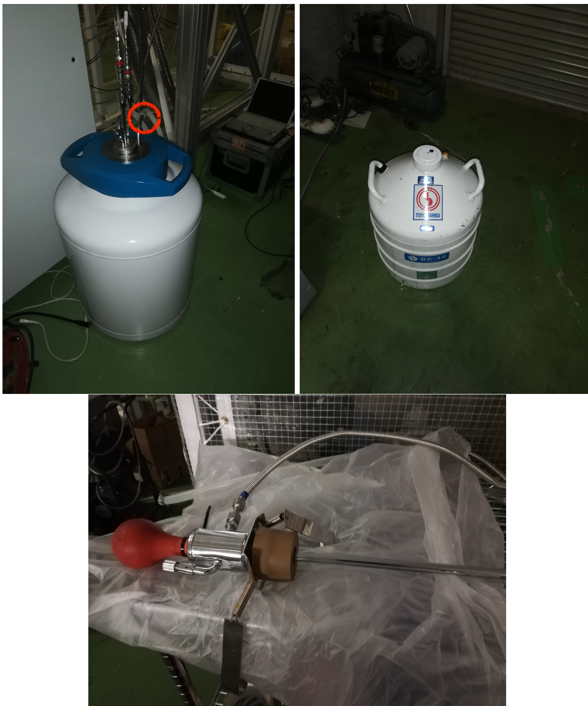
Figure 4.1: Top left: Liquid nitrogen dewar and cold trap. Red-circled indicates the position of ventilation port that is used for refilling; Top right: Liquid nitrogen dewar used for transport and refilling; Bottom: liquid nitrogen transfer tube used together with the dewar on the top right.
